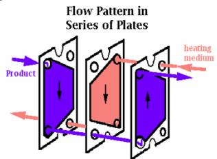
A plate type heat exchanger consists of a series of separate parallel plates forming thin flow pass. Each plate is separated from the next by gaskets and the hot stream passes in parallel through alternative plates whilst the liquid to be heated passes in parallel between the hot plates. To improve heat transfer the plates are corrugated.
