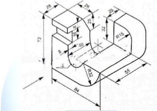
**4.** Figures show the isometric views of machine components and their view from the front, the view from above and the view from the right. Arrow indicates the direction to obtain the view from the front. Draw the orthographic views of the same. (10 x 2)
