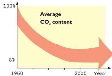
Increased welding parameters and reduced CO<sub>2</sub> content in the shielding gas leads to higher deposition rates and welding speeds. The drawback is that more ozone is formed.
