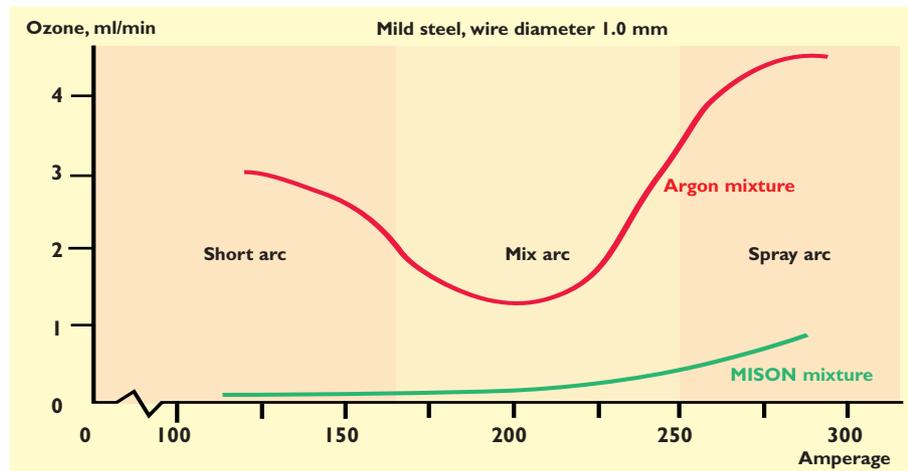
Ozone-emission. GMA welding with argon mixture and argon mixture with 0.03% NO. Compare diagram in section 3.3. Note the contrast between ozone and fume formation.
