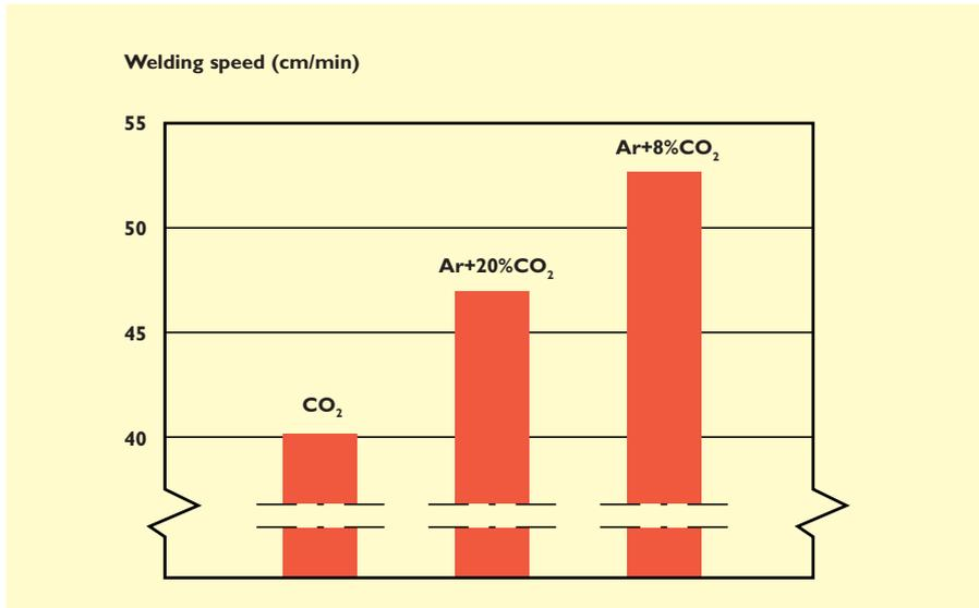
Example of welding speeds for fillet joints using different shielding gases. 4 mm throat thickness, 6 mm plate thickness, mild steel, wire diameter: 1.0 mm, wire feed speed: 12 m/min.
