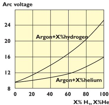
How different shielding gases affect the arc voltage in GTAW. Helium and hydrogen give more heat to the process which improves penetration and welding speed.
