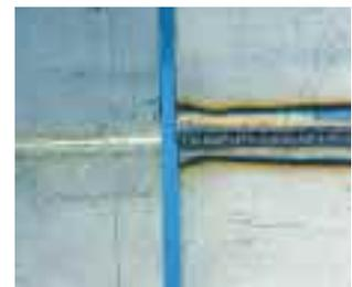
To the left: root side protected by argon-hydrogen mixture. To the right, no root protection.
