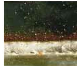
More  $\text{CO}_2$  creates increased and coarser spatter. Removal of spatter increases cost.
