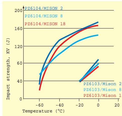
Impact strength for different types of shielding gases and filler metals.
