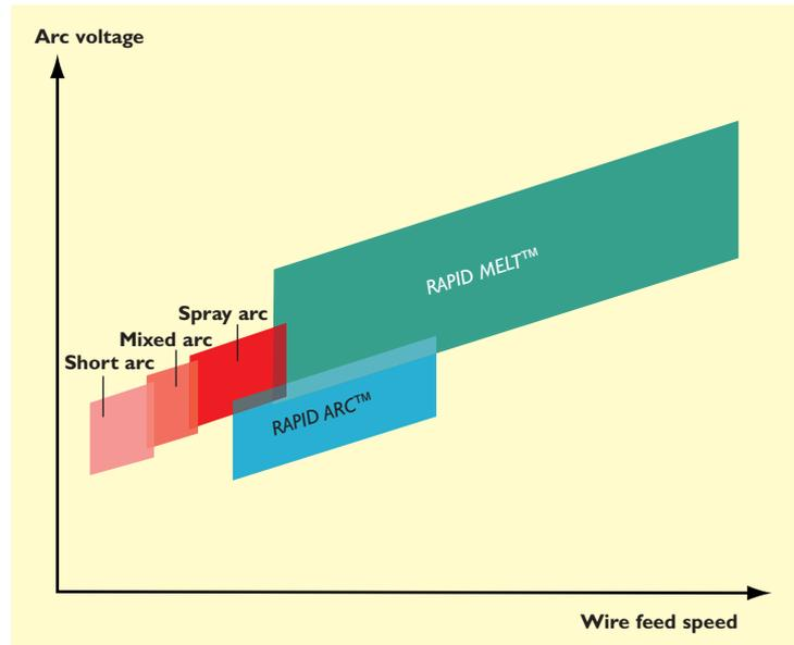
This is the thinking behind a concept for high-productivity welding developed by AGA. The concept comprises two welding procedures: RAPID ARC™, which aims at raising the welding speed in most plate thicknesses, and RAPID MELT™, which raises the deposition rate, primarily in the welding of heavier metal (e.g. 15 - 20 mm in thickness).
