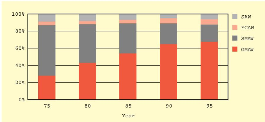
**Relative weld metal consumption per process in Western Europe 1975-1995. GMAW has developed because of its high deposition rate, the improved working environment, the lower total cost and the suitability for mechanized processes.**
