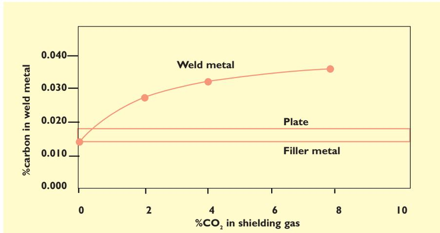
Carbon pick-up in austenitic weld metal with different CO<sub>2</sub> additions to the shielding gas is usually not a problem.
