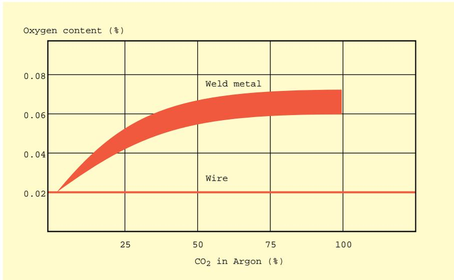
The influence of the shielding gas composition on oxygen content in weld metal. Higher oxygen content in the weld metal means more and coarser oxide inclusions. These may impair the strength of the weld metal.
