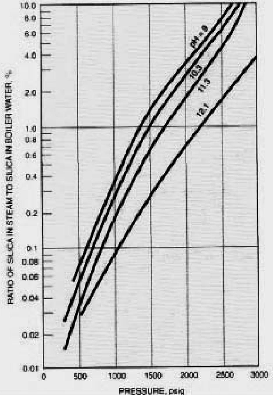
*Maximum boiler water silica allowable to maintain less than 0.02 ppm silica in the steam*
