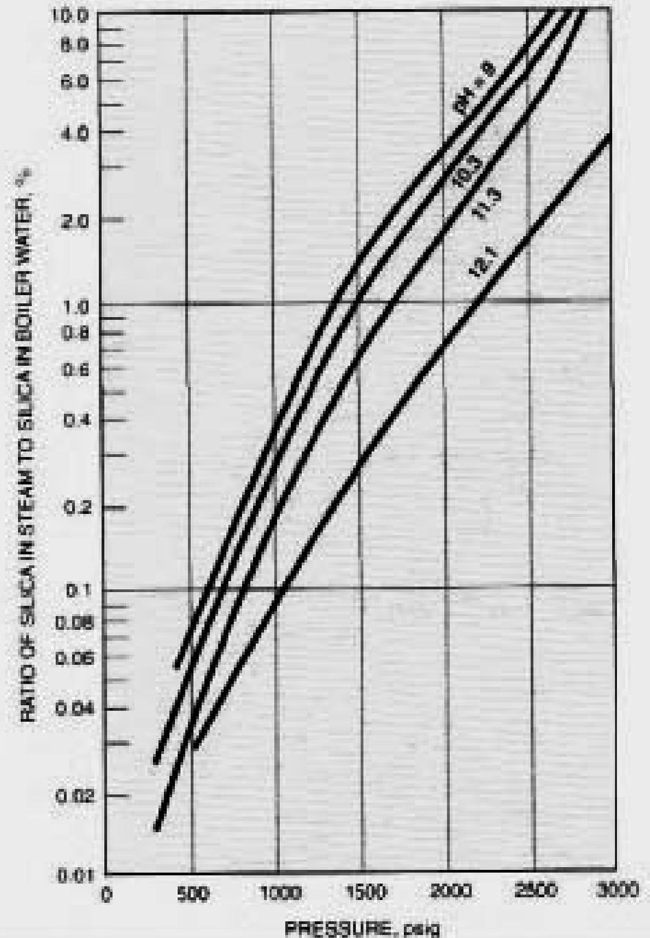
This ratio depends on water pressure and boiler water pH. The values of the ratio increases with increasing pressure and decreases with increasing pH. The effect of the pH becomes greater as higher pH values (from 11.3 to 12.1).
