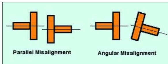
Figure 1. Diagram of shaft offset and angular misalignment
