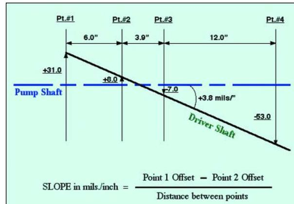
Figure 2. Angular misalignment calculation
