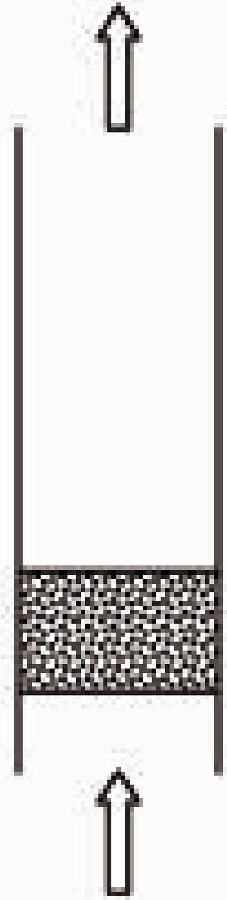
If the upward flow is very large, the bed mobilizes pneumatically and may be swept out of the process vessel. This is pneumatic transportation.
