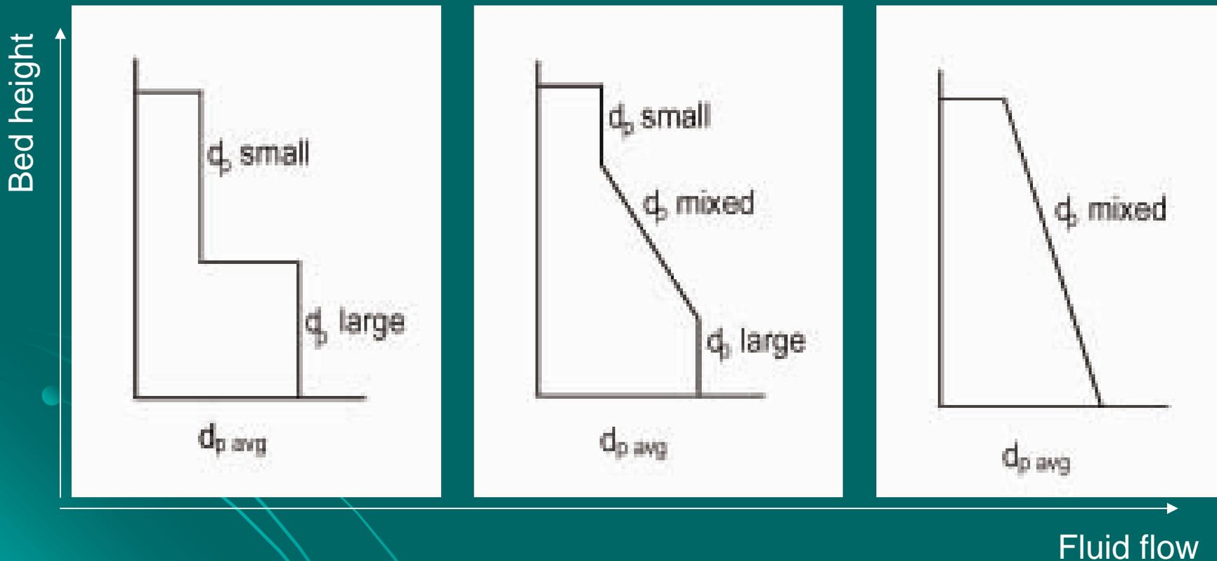
Particle segregate across the bed height as function of fluidizing gas flow rate.
