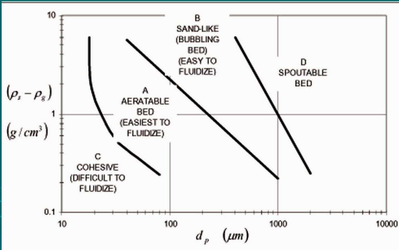
He categorized his observations on fluidization of different solid particle size versus the relative density difference between fluid phase & the solid particles. He identified four regions in which the fluidization character can be distinctly defined.
