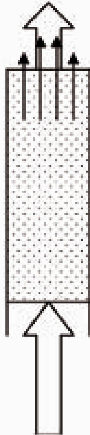
At an intermediate flow rate, the bed expands and is what we call an expanded state. In this state, the particles have a free distance between them. They are supported by the drag force of the fluid.
