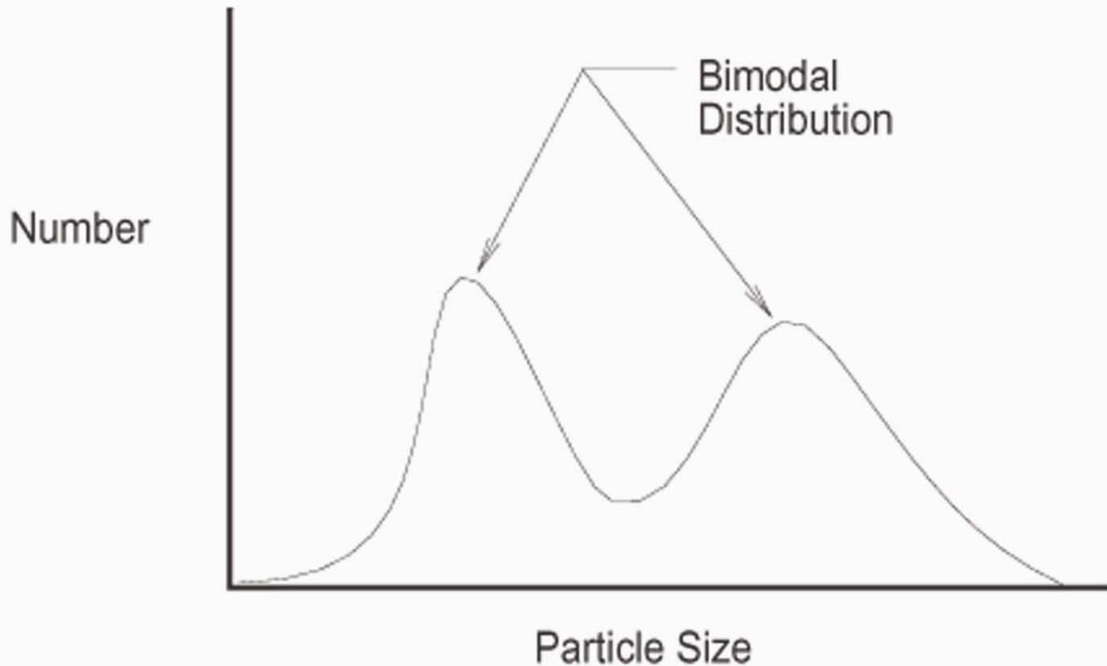
Bimodal distribution of particles leads to two different fluidization velocities. Poor performance is often the result of this situation.
