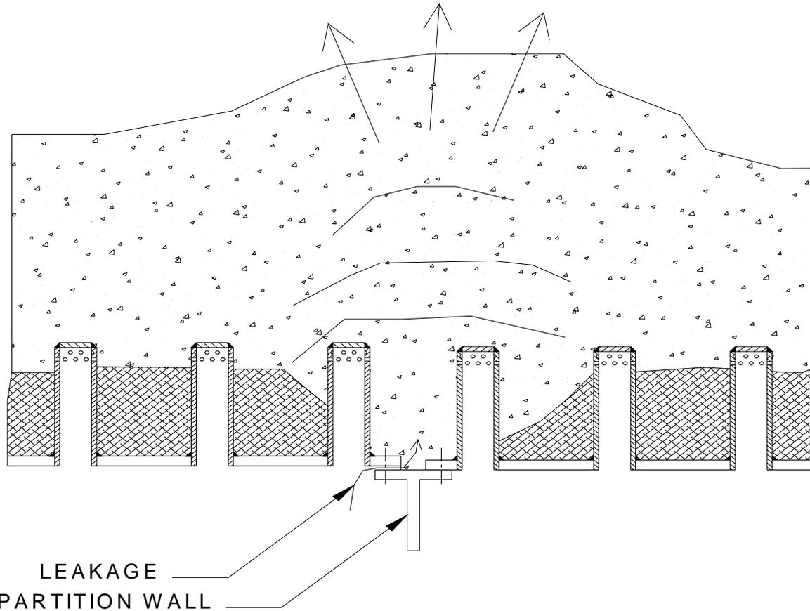
FIGURE 11: LEAKAGE BETWEEN SUPPORT FRAME AND DP PLATE
