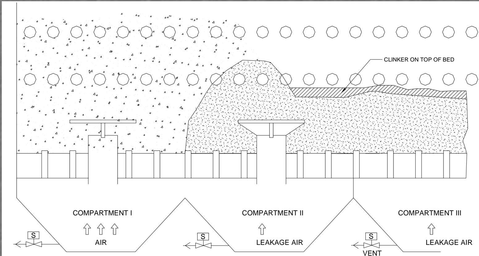
FIGURE 7 : FUEL SPILLAGE AND LEAKAGE AIR IN IDLE COMPARTMENT CAUSING CLINKERS
