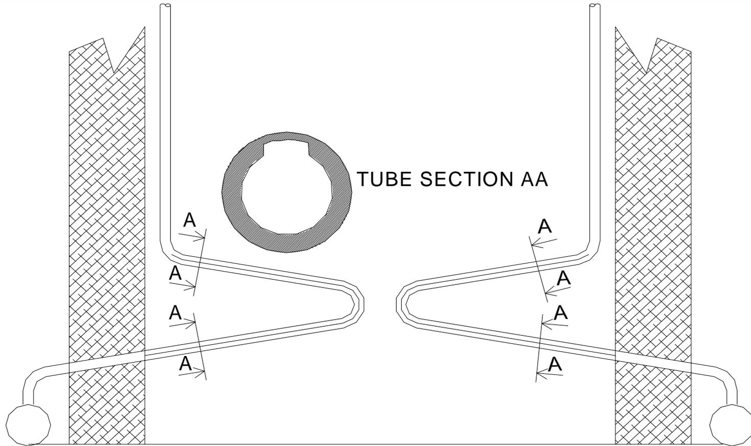
**FIGURE 5. CAUSTIC GOUGING ATTACK IN IDLE COMPARTMENT**
