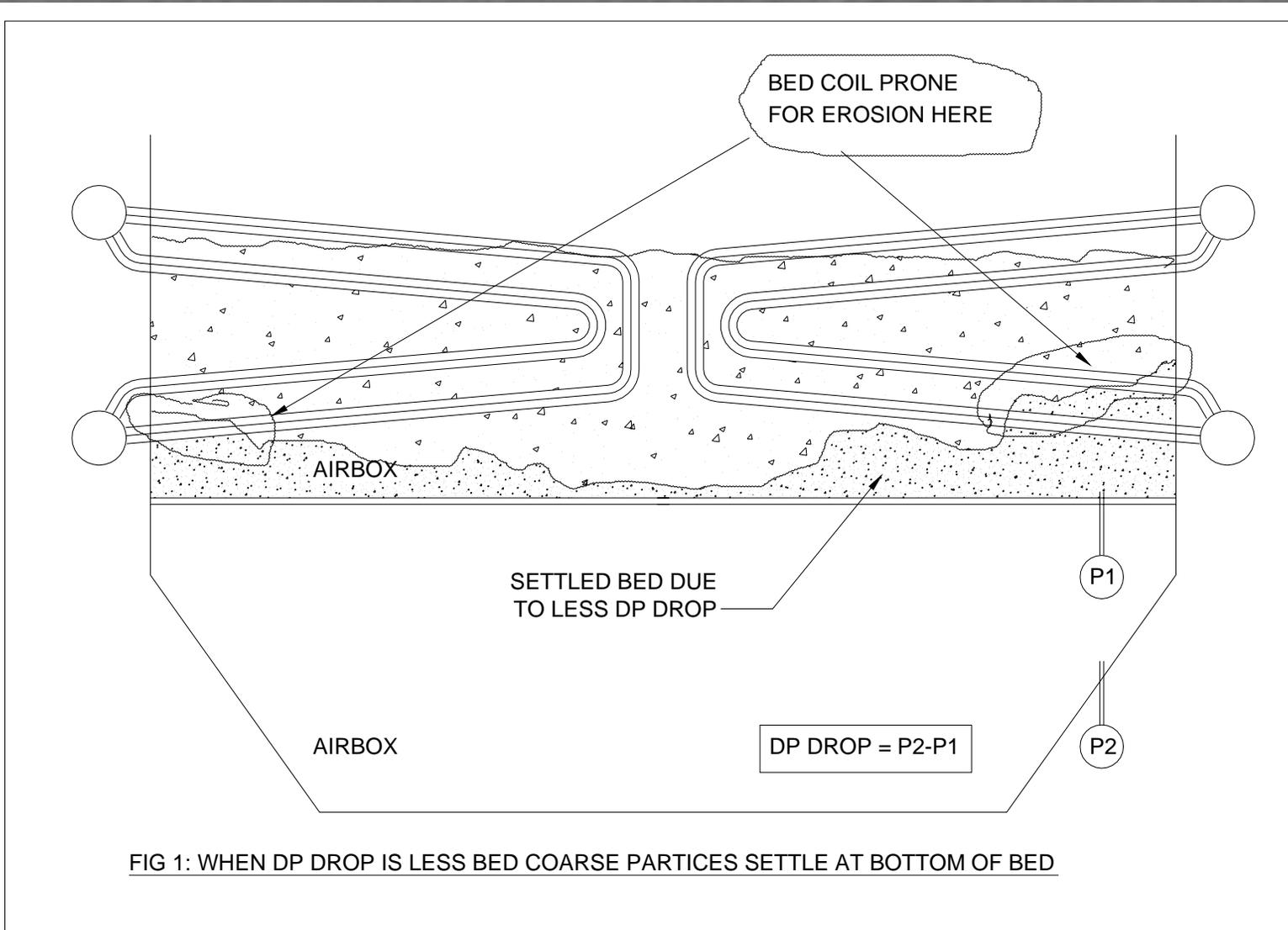
FIG 1: WHEN DP DROP IS LESS BED COARSE PARTICES SETTLE AT BOTTOM OF BED
